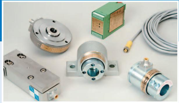
Cleveland-Kidder Ultra Line Load Cell Systems, consisting of load cell, amplifier and cable, provide better performance than competitive load cells by increasing the operating tension range from 8:1 to 40:1. (This means that a 50 lb. (222 N) Ultra Line Load Cell accurately measures from 1.25 lbs. (5.5 N) to 50 lbs. (222 N) of tension when used with an Ultra Line Amplifier.) Industry standard transducers currently measure tension ranges of only 8:1 to 16:1.
